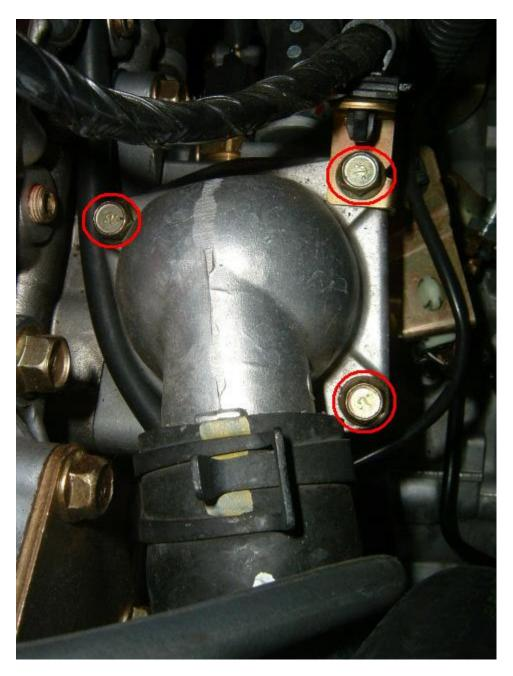
Pull the old thermostat out and replace it with the new one (pay attention to its orientation). Clean both sides of the housing and keep them free of coolant. Put a bead of Ultra Gray RTV around the upper housing and reinstall bolts (84  $\pm$ 13 in-lbs). Reinstall the intercooler piping and clamps (53  $\pm$ 1-9 in-lbs).
